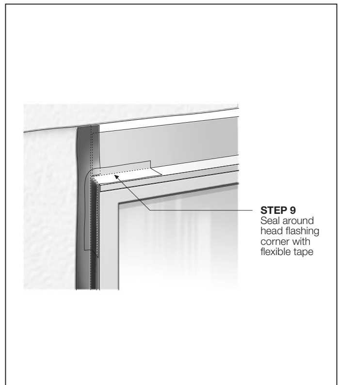
FIGURE 38 INSTALLATION OF WINDOW
