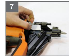
Reassemble tool, attached magazine to nose, replace cap screws and Nylock nut. Tool is ready to use.
