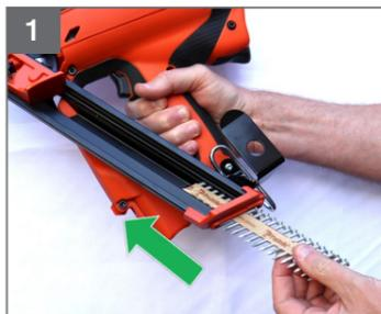
Slide nail strip into back of Magazine
