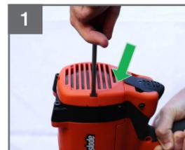
Use a flat bladed screw driver to remove cap
