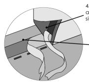
45 mm wide clear integrated adhesive tape on the underside of the membrane.
