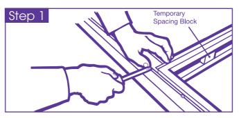
Step 1. Fit and screw the head track assembly to the cavity pocket using the 6 x 12mm countersunk screws. Do not remove the temporary spacing blocks until the wall sheeting has been completed.
