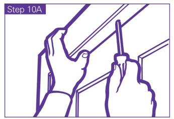
Step 10A. Screw in place the removable fillet using  $4 \times 35 \text{mm}$  screws through a white snap cap base. Finish off with supplied snap caps. Refer to Steps 10A, 10B and 10C.
