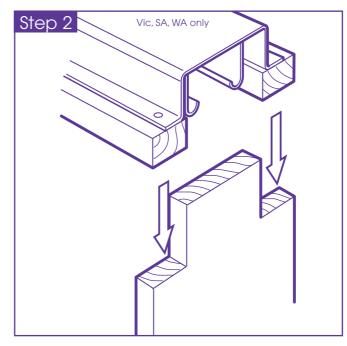
Step 2. Screw/nail the closing jamb to the head section, fixing through head timber into closing jamb stile.
