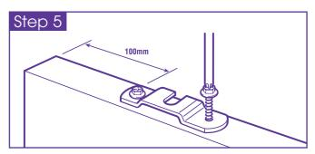
Step 5. Attach the door support brackets to the top of the door using the 4 x 30mm hex head screws, 100mm in from each side.
