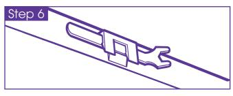
Step 6. Attach the spanner storage clip to the top of the door using the 1 x 15mm countersunk screw.
