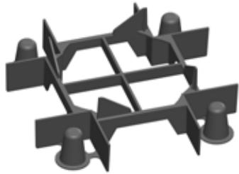
A highly effective, time-saving design that ensures the StyroPods are secure and held in place for increased stabilisation during the concrete pour. The StyroPod slots into the lugs located at each corner of the 4 way interlock, holding the pods tightly in place to guarantee a uniform concrete flow. The unique 4 way interlock design also allows for double-stacking of pods. Available in 110mm and 100mm.
