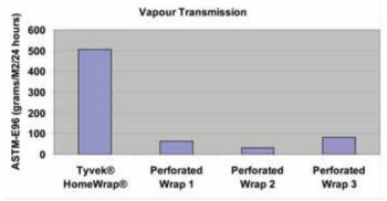
Not only do perforated housewraps allow moisture to pass through, they also slow the drying process, because the product can only breathe at these specific locations. Tyvek® HomeWrap® has a high vapour transmission rate, as measured under ASNZS 4200.1 Tyvek® HomeWrap® has very low vapour barrier properties.
