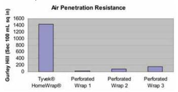
Tyvek® HomeWrap® has higher air resistance than perforated housewraps.
