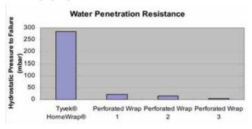
The ability of a housewrap to hold our bulk water is one of the most basic and important requirements of any weather resistant barrier. DuPont Tyvek® HomeWrap® has over 13 x Greater water holdout than perforated housewraps, as tested in accordance with the Hydrostatic Head Test (AATCC-127). Tyvek® HomeWrap® passed the high duty water holdout requirements ASNZ 4201.4
