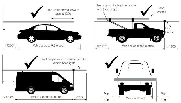
\*Rear projection may exceed 1200mm where the total length of the loaded vehicle does not exceed 12.5 metres and the rigidity of the product permits.
