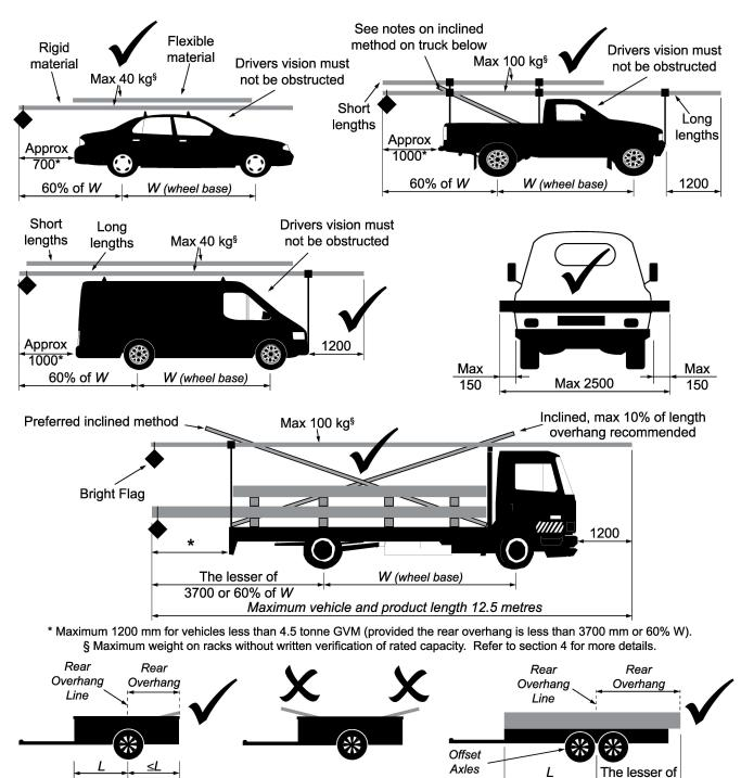
The rear overhang of a trailer must be the lesser of the front load carrying area or body ahead of the centre of the axle group (L) and 3.7 m. No forward or rearward overhangs for standard box trailers. *(Exceptions in QLD, WA & SA due to their definition of L)*
