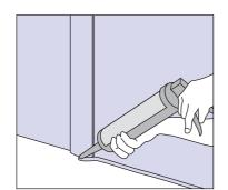
11 Continue this process to fix panels around each wall and seal gaps at the base of each panel using silicone sealant.
