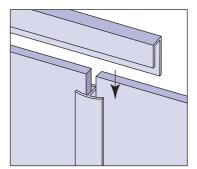
12 Upper and lower edges may also be finished using end caps. Should this joiner be used, ensure all lengths of vertical sheet joiner finish 11mm short of edges. A bath mould is recommended for the lower edge of panels butting against a bath rim.
