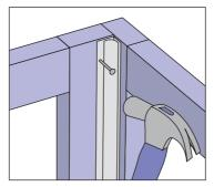
**4** Begin in one corner by nailing or stapling an internal corner joiner to the timber frame.
