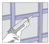
**5** Apply a 5mm bead of adhesive to the face of each timber batten that the first panel will be applied to.
