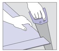
2 When cutting straight lines use a fine tooth handsaw and always cut with the panel face up. If using a fine tipped tungsten machine saw ensure the panel is face down. Sand or hand plane cut edges to achieve a smooth finish. Use a fine toothed hacksaw to cut your colourmatched joiners to size.
