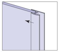
**8** Slide the panel into the joiner and position the panel carefully. Fix the next joiner to the free edge of the panel and press the sheet into its final position.
