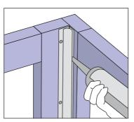
**7** Place a bead of silicone sealant along the inside of each joiner (internal corner, sheet joiner, etc.) to create a 3mm expansion gap.
