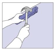
**9** Use a wood block wrapped in a soft cloth to work across the surface of each panel, tapping the block gently with a hammer to ensure the adhesive on all battens makes contact with the panel, particularly around the edges.
