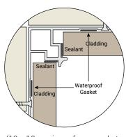
(12 x 10mm inner foam gaskets optional, alternative sealant option)
