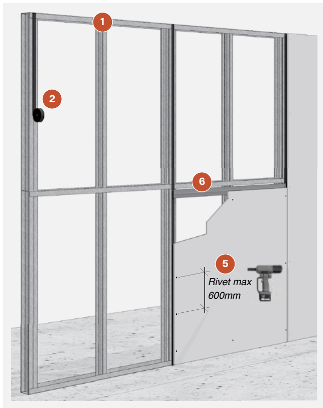
FIGURE 7.29 Exposed Screw or Rivet Fixing to Steel Frame
